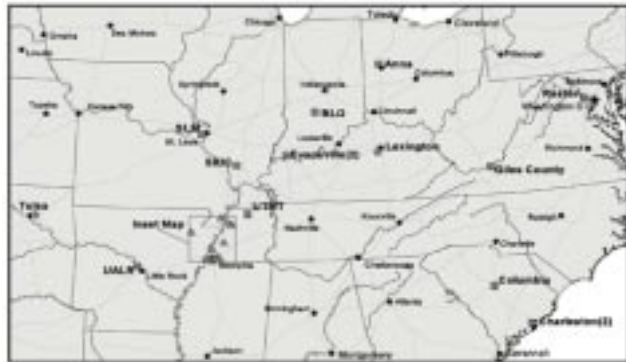
Figure 3: ANSS-MA station map. While other regional and national network stations will be designated as ANSS sites, current ANSS-funded stations include 12 installed in FY01 (4 free field, 8 urban reference) and 15 proposed for installation in FY02.
